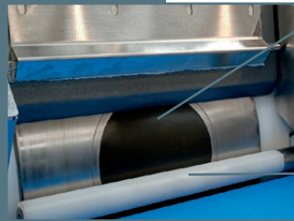
Supplementary lubrication system for drum with tap Lubrificazione supplementare per tamburo con rubinetto
